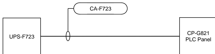
Figure 7-3: Instrument Cable Identification Example – Identified Equipment
